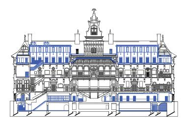
View on the restored front façade seen from the Grand Place. As the façade Axonometry and floor is an iconic image, it was plans showing in blue the central existing and new important to preserve the view completely. The new vestibules, added on the interventions are therefore second floor as a continunot visible from the Grand ation of te existing. A new Place circulation core is located Image ©Stijn Bollaert in the south-west corner.
