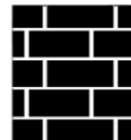
Sandstone-limestone piece measuring 80x20x40cm with M-5 mortar joints.
