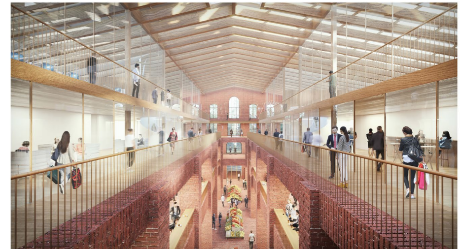
The diverse functions of Building 1 are united by a central atrium and covered by a top-lit wooden roof, reconstructed to its original geometry.
